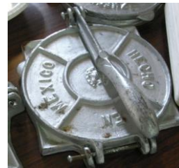
▲ dough rolling-out machine, kneading maize flour to make dough for tortilla.
